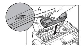
7 Insert the toner cartridge so that the guide (A) on the left side of the toner cartridge fits into the groove inside the machine and slide it down parallel to the guide.
